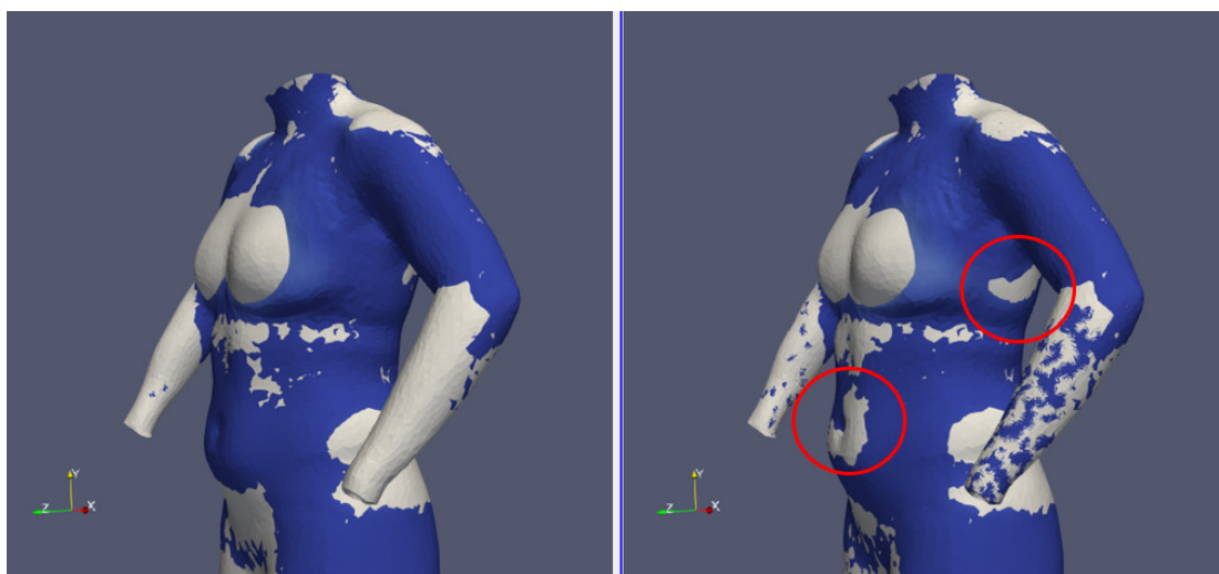
Figure 14: The body shape before wearing the FPV (white) is superimposed on the body shape compressed by the FPV (blue). Therefore, visible white areas highlight those that were pushed in by the armour. The left image shows the “comfortable” strap condition and the right image shows the “tight” strap condition. The greatest differences, highlighted in red, appear to be in the lower abdomen and sides, with additional inward displacement of soft tissue in the tight condition.
