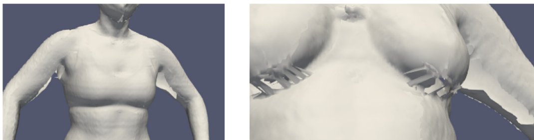
Figure 2: Most 3D scanners, including the one used by DRDC, have difficulty scanning concave regions and occluded areas. These lead to holes and spurious geometry.
